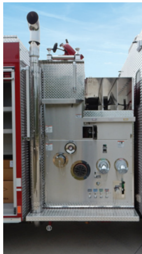
Shown with a traditional pump house configuration.
